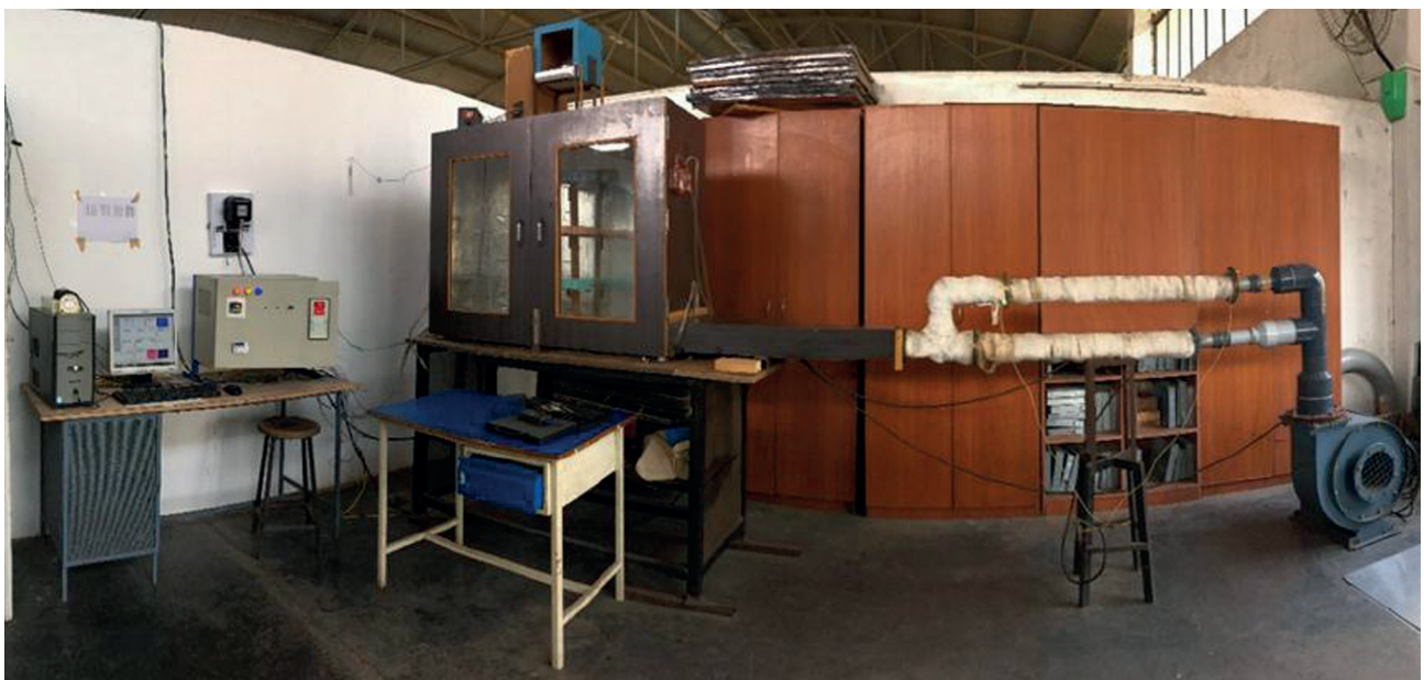
Figure 1. Air dryer experimental setup.
